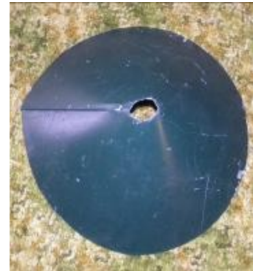
Above is the finished product for the cone guard. It is mounted on a tee post.
